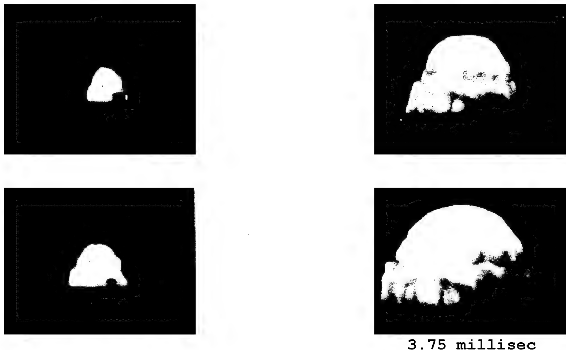
Fig. 2.1, Kerr cell camera photos of fireball emerging from far side of ship. Bows of ship are visible as dark region in the lower right of the fireball.
